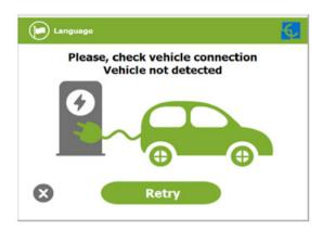
**H –** Almost all vehicles cannot charge if the shift lever is not in parking mode position. This situation can be detected for the Charging Station and it will be displayed by HMI as "Please, check vehicle shift position, put in parking mode", after pressing over "Retry" button.
